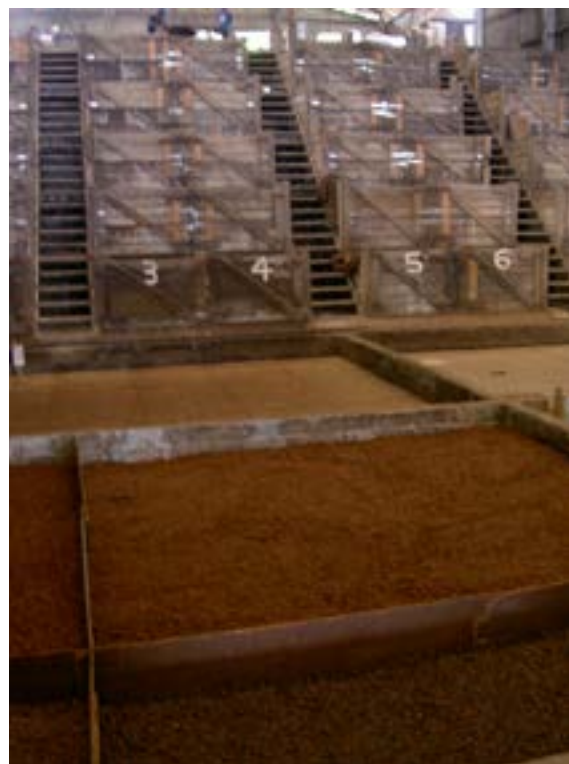
Figure 12.9 – Multi-tiered fermentation boxes in a large commercial fermentary; 5 tiers allows 5 turnings. Large forced air driers with diesel heating in the foreground (Courtesy of NGIP-Agmark, Kokopo)
