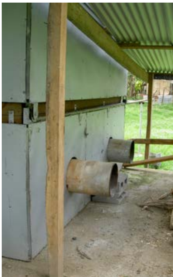
Figure 12.21 – A well-constructed cocoa drier with a double wood-fired kiln and galvanized iron cover that can be rolled off on rails to expose beans for sun drying
