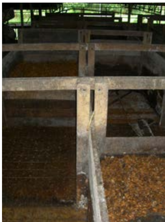
Figure 12.1 – A row of large fermentation boxes showing how the side boards are held in slats and can be removed to adjust the size of boxes or facilitate turning
