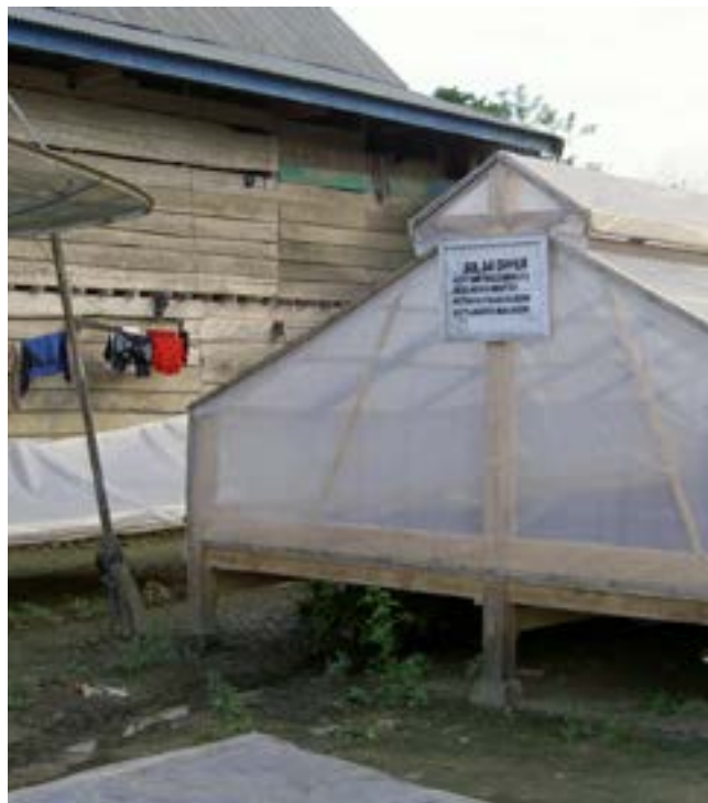
Figure 12.14 – Sun drying of cocoa with simple plastic-covered structure - note the vent in the roof that allows air to be drawn up through drying beds and the plastic sides that can be rolled down to cover the beans during rain
