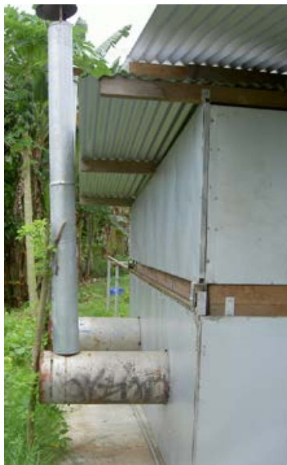
Figure 12.21 – A well-constructed cocoa drier with a double wood-fired kiln and galvanized iron cover that can be rolled off on rails to expose beans for sun drying
