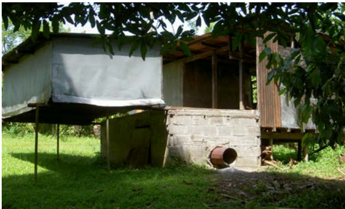
Figure 12.20 – Wood-fired kiln with galvanised iron cover rolled off to expose the drying rack
