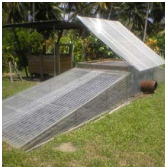
Figure 12.17 – Photos of combined solar/wood-fired kiln drier showing the polycarbonate sheets covering the black rock beds to guide hot air up through the drying rack that is protected by a polycarbonate roof that can be rolled off on rails to expose the beans; the wood-fired kiln can be lit during rain
